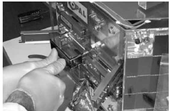
Figure 2.6 Loading a Picosat into OPAL
