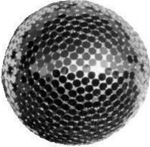
Figure 7. The First Starshine Satellite to be launched from the Space Shuttle in Spring 1999. The sphere is 19 inches in diameter.
