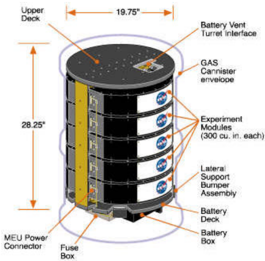
Figure 5. The NASA Space Shuttle Student Experiment Module
